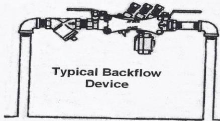
Diagram of typical backflow device.
